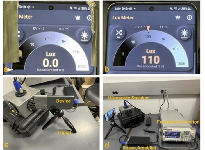
Fig. 7. **Occluded and Open Camera Setup.** Occluded camera is on the left, open camera is on the right. An on-device application is used to record the experienced lack of sensor irradiation by the rear camera. Lux is a unit of sensor illumination, and a lux of  $\approx 0$  implies the sensor is not receiving enough light to change the reading for the on-device application.
