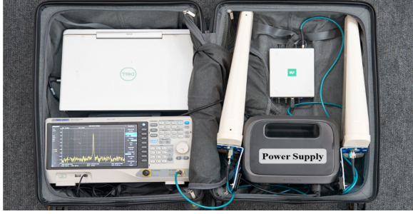
Figure 17: The portable prototype is integrated into a suitcase. Key components include an antenna array, an SDR transceiver, a spectrum analyzer, a laptop, and a portable power supply.
