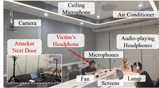
Figure 15: An office eavesdropping setting with diverse interference from multiple ceiling-mounted and desktop electronics. The injection-induced leakage remains robust to interference.
